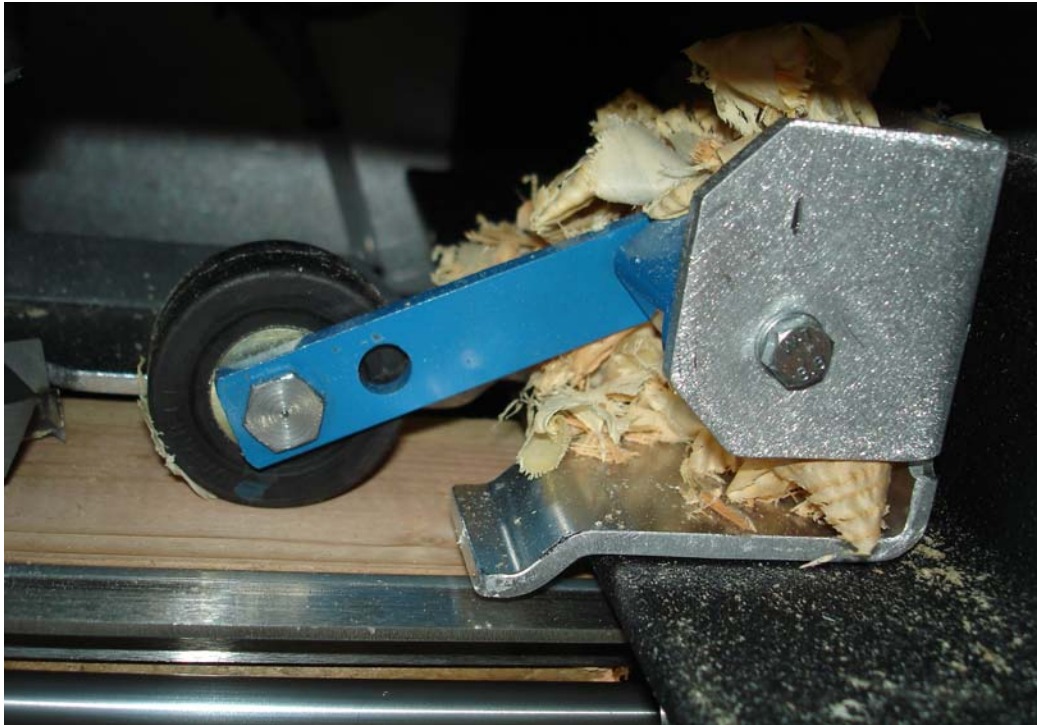
Photo 7-3 Friction Wheel Adjustment
