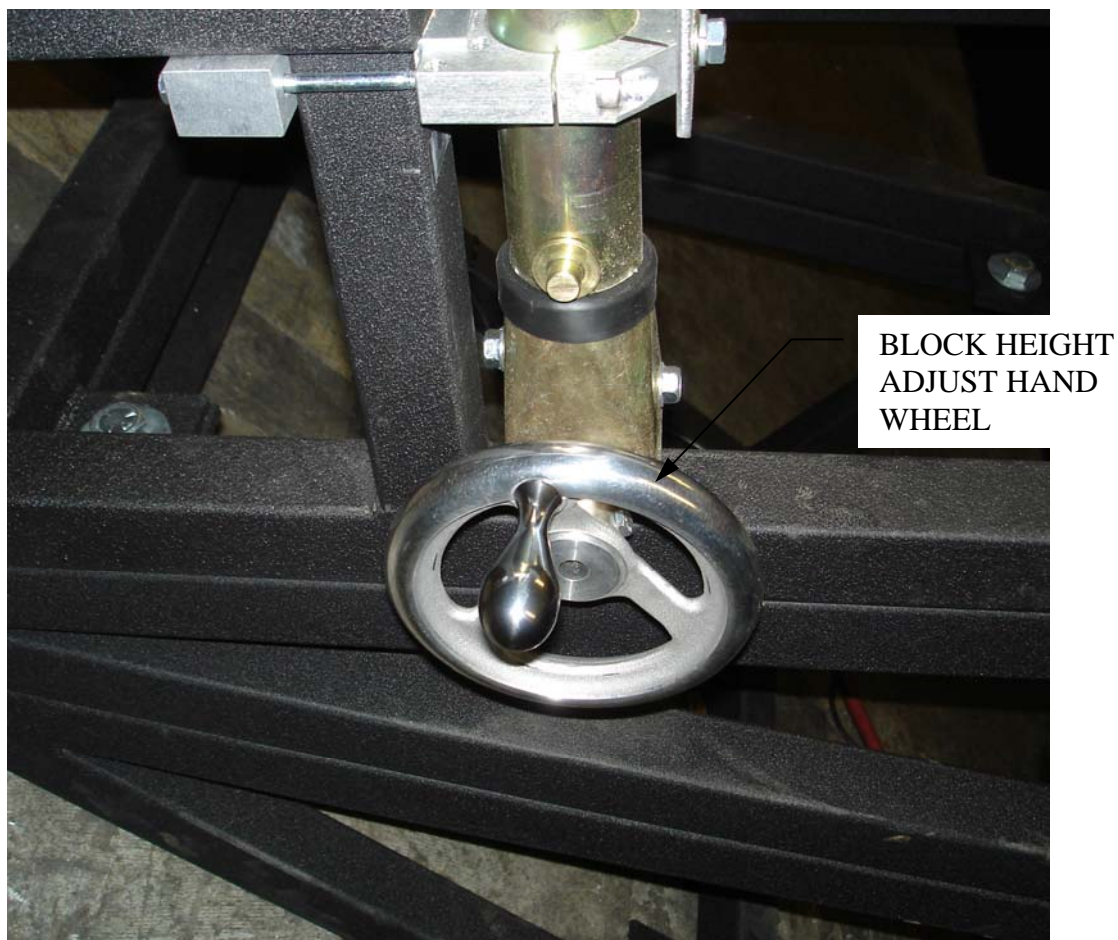
Photo 3-6 Model VBD Auto-Feed Block Height Adjust Hand Wheel
