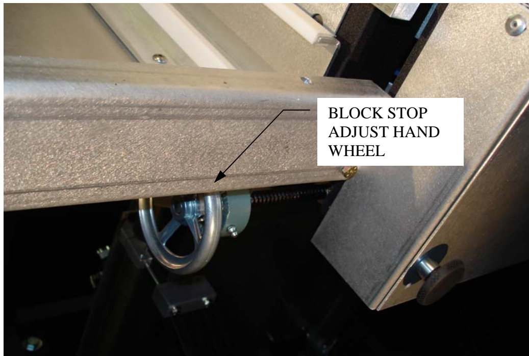
Photo 3-7 Model VBD Auto-Feed Block Stop Adjust Hand Wheel
